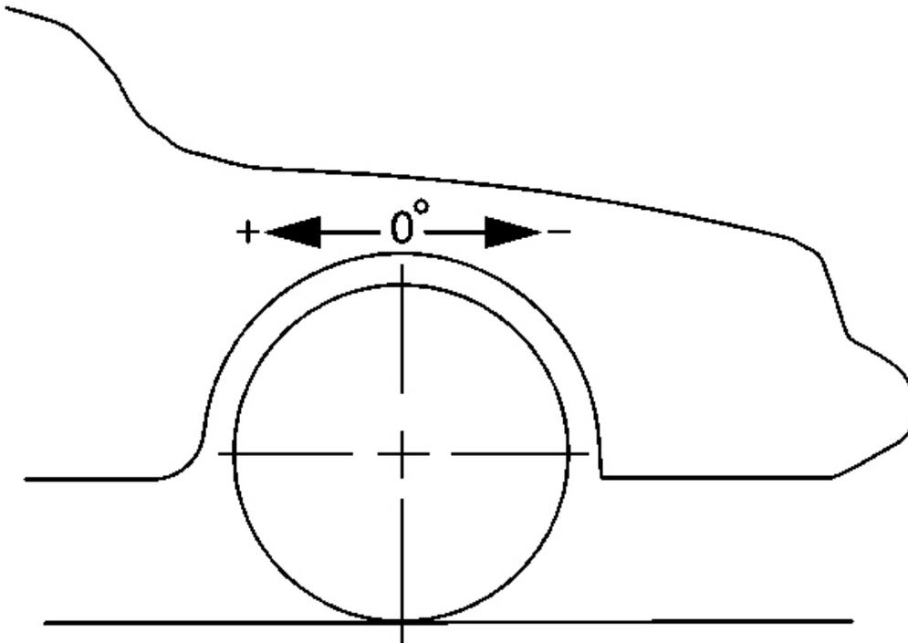
**Fig. 5: Illustrating Caster Angle**
