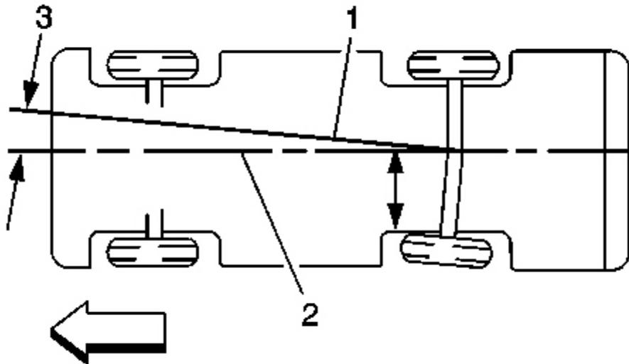
**Fig. 8: Illustrating Thrust Angles**
