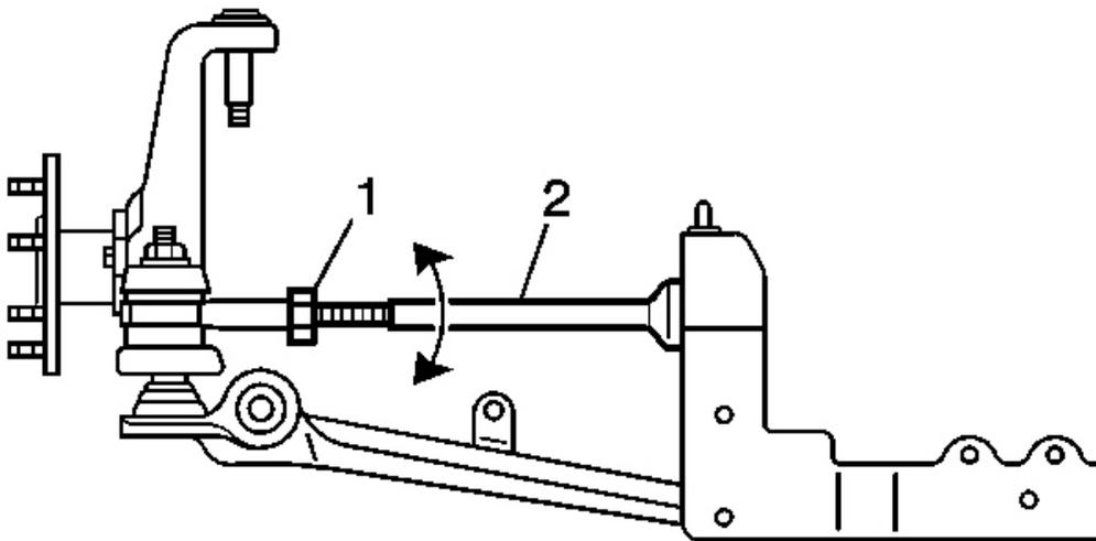
**Fig. 4: Rear Suspension Adjustment Link Lock Nut & Inner Tie Rod**
