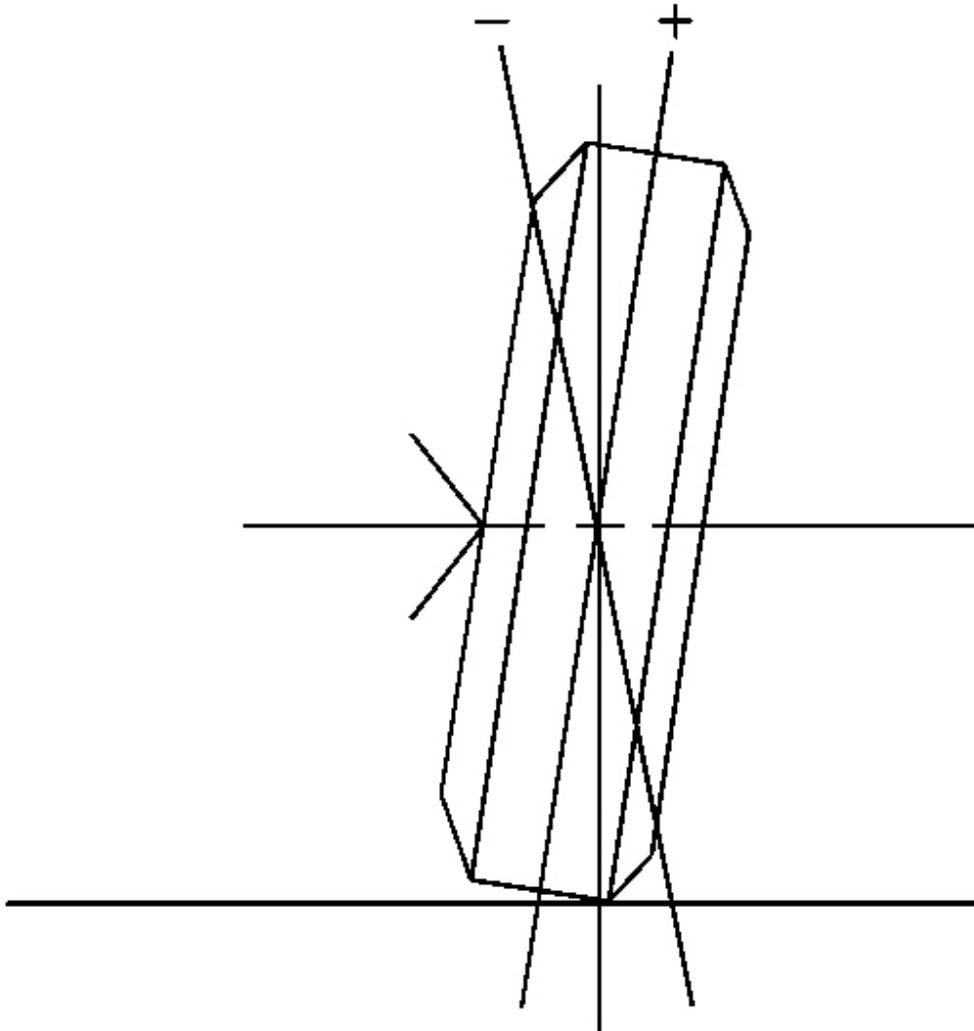
**Fig. 6: Illustrating Camber Angle**
